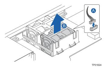
Figure 42. Removing a Power Supply Fan Module
